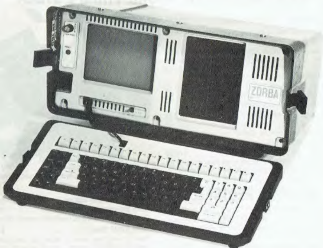
The Zorba portable computer bears more than a faint resemblance to the Osborne, although it's a little smaller and lighter. At 10 kg, though, it's still a borderline 'portable' as opposed to 'transportable' computer.
